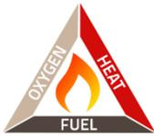
The triangle illustrates the three elements a fire needs to ignite: heat, fuel, and an oxidizing agent (usually oxygen). If one of these three is removed, the fire will be put out. In the middle of the fire triangle there is also a chemical reaction.
